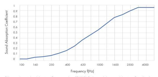
Table presents the practical sound absorption coefficients as according to ISO 11654. Graph presents third octave sound absorption coefficients (According to ISO 354 Measurement of sound absorption in a reverberation room.) The NRC rating is determined as the arithmetic average of the absorption coefficients measured by one-third octave bands centred on 250 Hz, 500 Hz, 1000 Hz and 2000 Hz. and rounded to the nearest 0.05.
