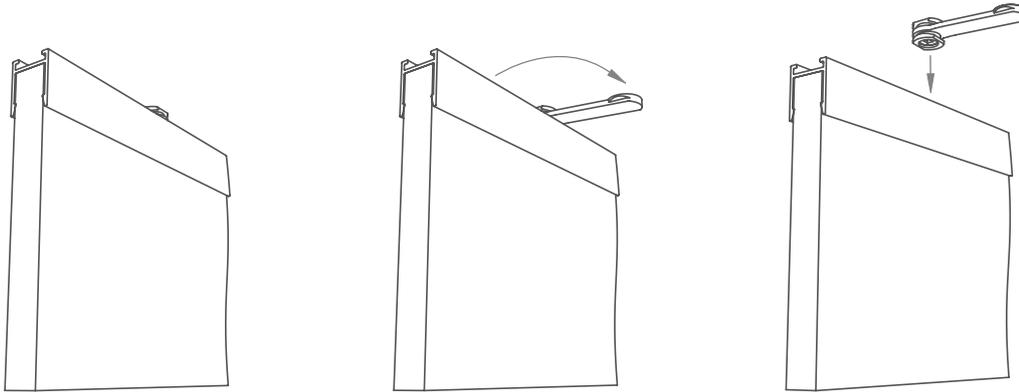
Locate the Frontier Connector clip, then using a Phillips head screw driver or flat object, carefully pop the Connector handle out of Channel space.
