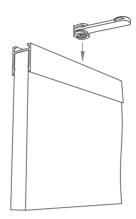
Once the connector clips are turned 90 degrees, the Frontier Channel can be disconnected from the ceiling.
