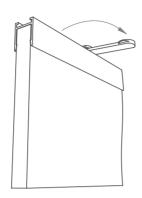
While taking the weight of the Frontier fin, turn the connector 90 Degrees.
