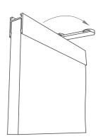
Whilst taking the weight of the Frontier™ fin, turn the connector 90 Degrees.
