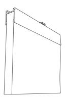
Locate the Frontier Connector clip, then using a Phillips head screw driver or flat object, carefully pop the Connector handle out of Channel space.
