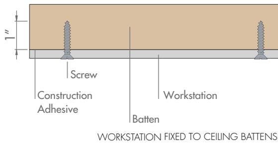
We recommend fastening Workstation panels from one side to the other to help avoid pillowing and sagging through the middle of the panel.
